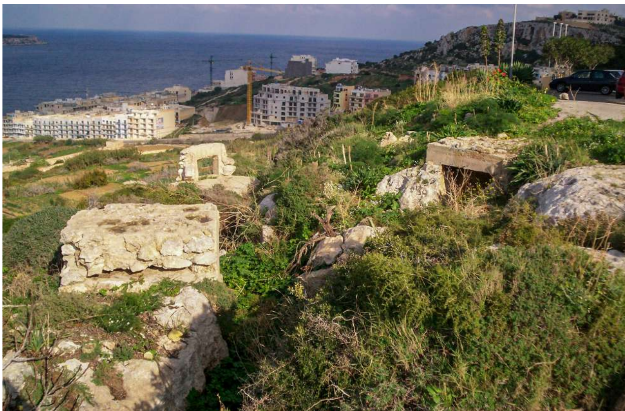
Part of the infantry trench and casemates for a Vickers 0.303-inch Machine-Gun and the entrance to the bunker from the same trench.
